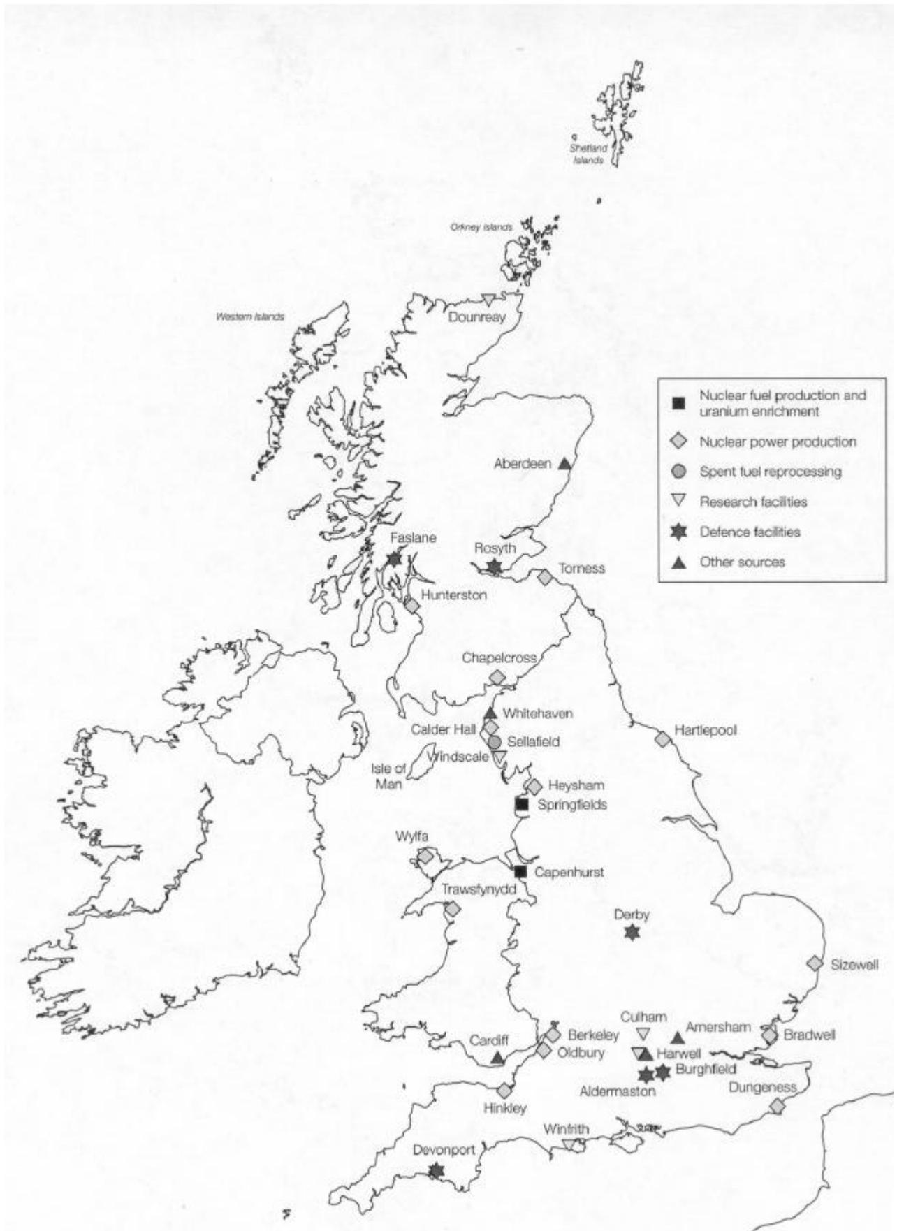
Figure 1.2 Location of principal sources of radioactive discharges in the UK (DETR, 2000)
