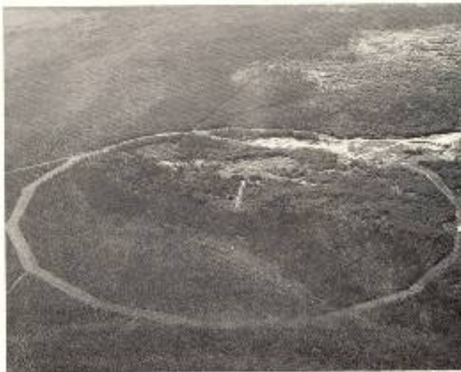
FIGURE 1. Field Irradiator - Canada (FIG) site. The fenced forest area, 1000 m in diameter and surrounded by a 1.5 m high fence, is located in southwestern Manitoba. Irradiation has continued at 19000 Ci for over 1000 hours.
