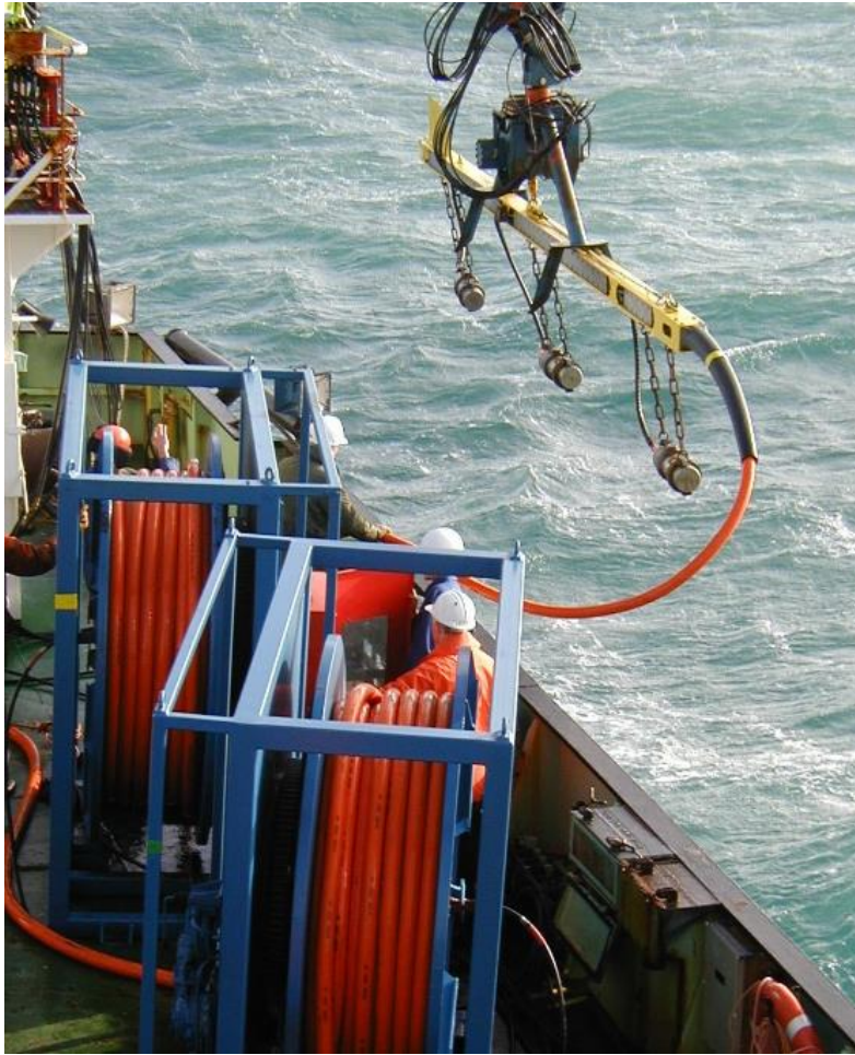
Airgun deployment during seismics operations
